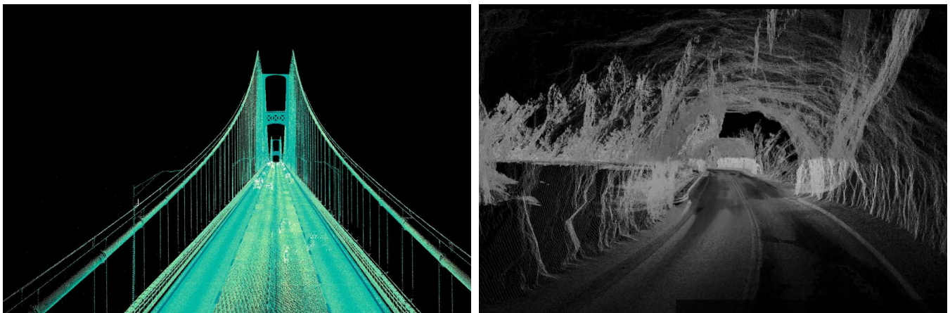
High-Precision 3D Data imagery of a bridge and tunnel
